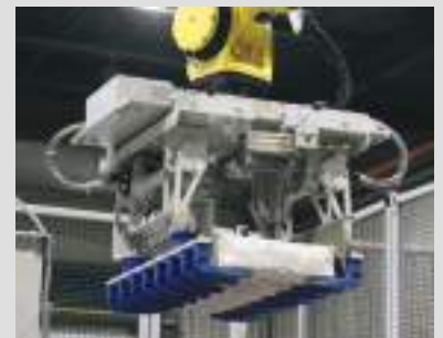
Finger gripper equipped with automatic bag width adjustment system.
