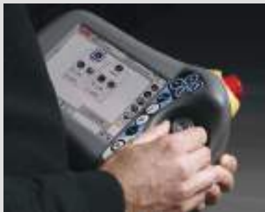
Color teach pendant used as main interface on standard cell
